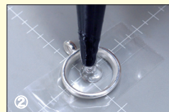
② Turn it over and pour UV resin to make first layer in about 1 mm thick.
