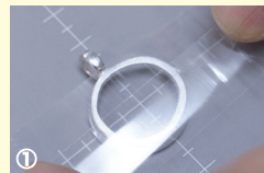
① Seal the bottom of the finished silver frame with a sticktape to hold UV resin.
