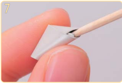
Expand the hole gently with a toothpick to thread the silver wire. *Do not open the hole up too much so as not to lose the desired shape and create cracks.
