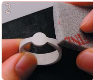
Make a 1.5mm thick flat ring with a round stage using Clay Type, fix the shape with a red sponge sanding pad (#320-600), and fire the ring.
