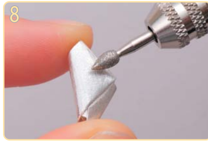
Fire (p.3) and polish all pieces with a stainless steel brush. Then, make a matte finish to 2 large, medium and small pieces with sponge sanding pads or the diamond point.
