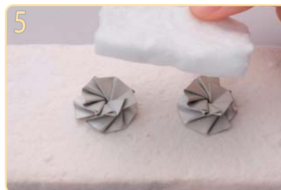
5 Place 2 pieces on a fiber board, and cover with some fiber cloth gently. Fire at Paper Type's preferred firing condition.
