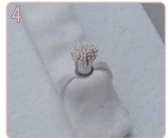
Make a ring mandrel with some fiber cloth to help stand the ring, dry, and fire at 800°C/1472°F for 30 mins. *If firing at 850°C/1562°F for 20 mins, the petals will stick too closely and be difficult to open up.
