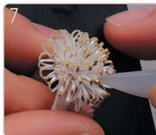
Support the petals with your fingers and burnish with an agate burnisher. Polish the ring band with a stainless steel brush and a red sponge sanding pad (#320-600).
